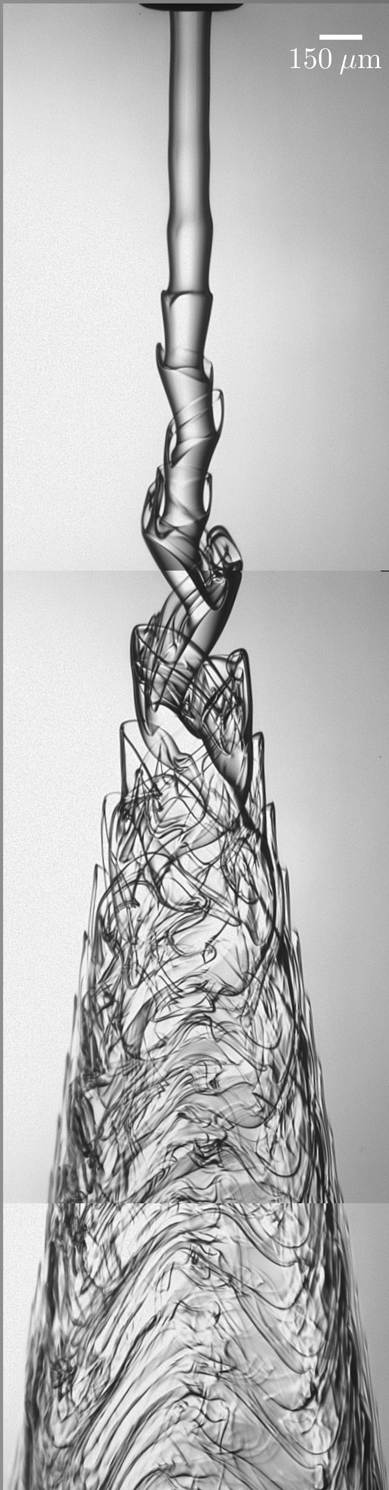
Newtonian jet (water + glycerol) is discharged in the background liquid in the bath, water: Re_j \equiv \rho V_j D / \mu \simeq 150 , kR_0 = 0.5 \rho / \rho_w = 1.1 , \mu / \mu_w = 3
